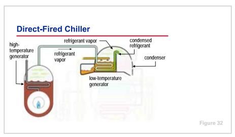
The example direct-fired chiller shown here employs the reverse-series flow cycle. In the **high-temperature generator**, the intermediate solution absorbs heat that is generated by the combustion process. Similar to the indirect-fired, double-effect chiller, this transfer of heat causes the refrigerant to boil and
